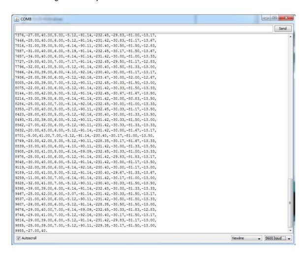
7. The data includes the time stamp (millisecond), 3 rotation rates, 3 accelerations, and 3 magnetic field strength. Turn the IMU board around to find out which data is which. After you understand the data, you can use Wireless MovSens 9DOF IMU for your own applications.
