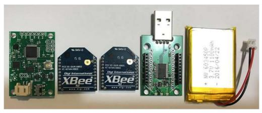
It is also highly recommended that you have an FTDI basic breakout (<u>Get it here</u>) and a miniUSB cable, for downloading Arduino program to IMU board through UART.
