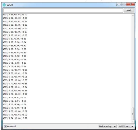
You can rotate the IMU board now and see the numbers streaming out on the serial monitor change. This suggests the firmware is working fine.
