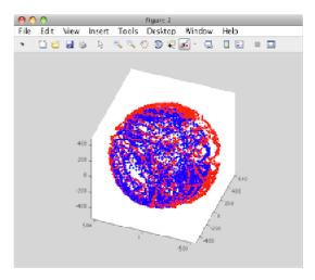
Another calibration example: Soft iron gives a sphere scaled and distorted into an ellipsoid.
